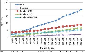
Figure 15: Performance of Word Count Job Using Panda-1GPU, Panda-24CPU, Panda-1GPU+24CPU, Mars-1GPU, Phoenix-24CPU on Delta Machine.
