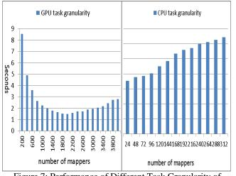
Figure 7: Performance of Different Task Granularity of Panda C-means Jobs on GPU and CPU.
