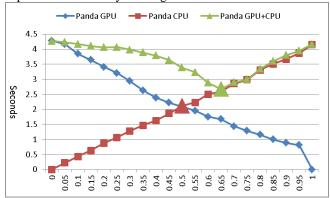
Figure 14: Effect of workload distribution on Panda wordcount jobs using 150MB text file on Keeneland machine. For Panda job only using CPU, the value X on x-axis means X percentage of work load is mapped to CPU. For Panda job only using GPU, the value X means (1-X) percentage of work mapped to GPU. For Panda job using both GPU and CPU, the value X means X percentage of work was mapped to CPU, and the remain (1-X) percentage of work is mapped to GPU.
