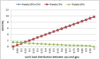
Figure 8: Effect of workload distribution on Panda C-means on GPU and CPU on Delta machine. For job only using CPU, the value X on x-axis means X percentage of workload is mapped to CPU. For job only using GPU, the value X means (1-X) percentage of work is mapped to GPU. For job using both GPU+CPU, the value X means X percentage of work was mapped to CPU, and the remain (1-X) percentage of work was mapped to GPU.
