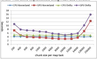
Figure 13: Performance of Panda Word Count with Different Chunk Sizes on Keeneland and Delta Machines.
