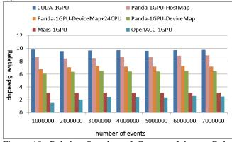
Figure 10: Relative Speedup of C-means Jobs on Delta Machine Using Panda-1GPU-DeviceMap, Panda-1GPU-DeviceMap+24CPU, Panda-1GPU-HostMap, CUDA 1GPU, Mars-1GPU, and OpenACC-1GPU, Using OpenMP 24CPU as the Baseline Performance.
