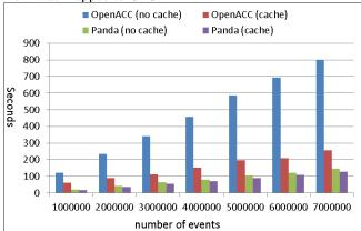
Figure 9: Performance of C-means jobs using Panda and OpenACC on 1 GPU with/without cache loop invariant data.
